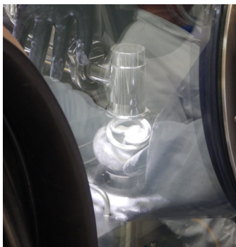
Figure 2: Agglomeration of test material when performing APCPPE tests
