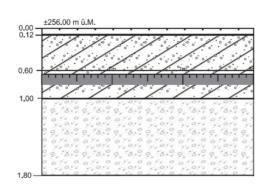
Different layers (road surface, roadbed, backfill of line, gravels or broken stone)
